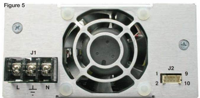
b. Conventional fan guards, fitted flush to the chassis, can create considerable air turbulence and noise. The custom-designed fan guard shown in Figure 5 is punched out of sheet metal and raised up to create a 4mm gap between the fan and the fan guard. This reduces fan noise by 4dB, a welcome improvement in many operating environments.
